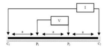
Figure 1. Wenner electrode configuration (Source: Loke, 1999)
