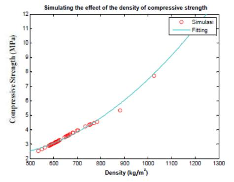
Figure 9. Simulation results of the effect of density on compressive strength
