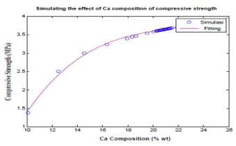
Figure 5. Simulation results of the effect of wt% Ca on compressive strength
