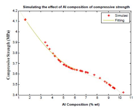
Figure 8. Simulation results of the effect of wt% Al on compressive strength
