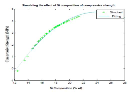
Figure 6. Simulation results of the effect of wt% Si on compressive strength
