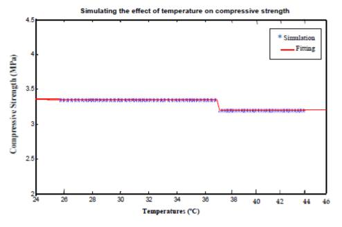
Figure 10. Simulation results of the effect of temperature on compressive strength
