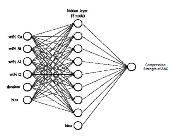
Figure-3. Artificial neural network architecture
