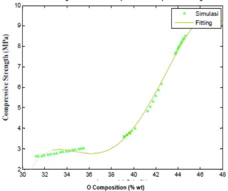
Simulating the effect of O composition of compressive strength
