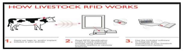
Figure 5: How livestock Radio Frequency Identification works? (Source: Datamars, 2015).
