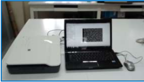
Figure 1. An HP scanjet (G3110) flat bed scanner coupled with a laptop computer
