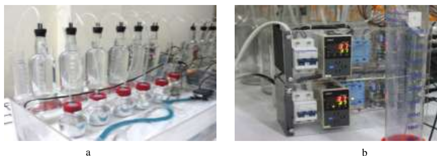
Figure 1. The experimental set-up include a water bath with reactors and gas collection bottles (a) and temperature controller (b)
