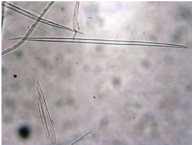
Fig.3. High magnification of date palm fiber
