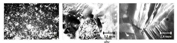
Fig.2. The microstructure of the alloy aged at 900<sup>o</sup>C 1250<sup>o</sup>C from pre-hardened, 1 min: a - x1000; b - x7500; c - x7000
