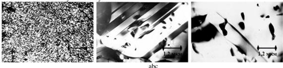
Fig.3. The microstructure of the alloy after quenching from 47CrNiMo 1250<sup>o</sup>C, 1 min. and aging at 1000<sup>o</sup>C: a - 5 hours, x450; b - 1 hour,x8500; c - 1 hour,x8500
