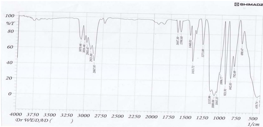
Figure (1) : FTIR spectrum of vinyltriallyloxysilane monomer.
