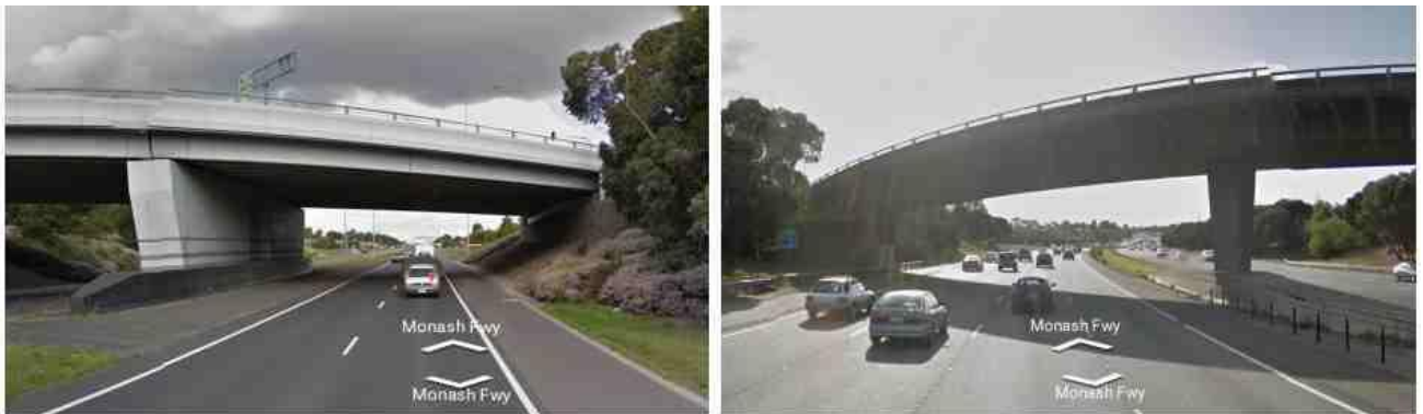
Figure 8: Example of the environments where speed outliers were generated on the test route No1 by the GPS receiver with 5° mask angle with speed differences 2.2 km/h (left) and 5.5 km/h (right)
