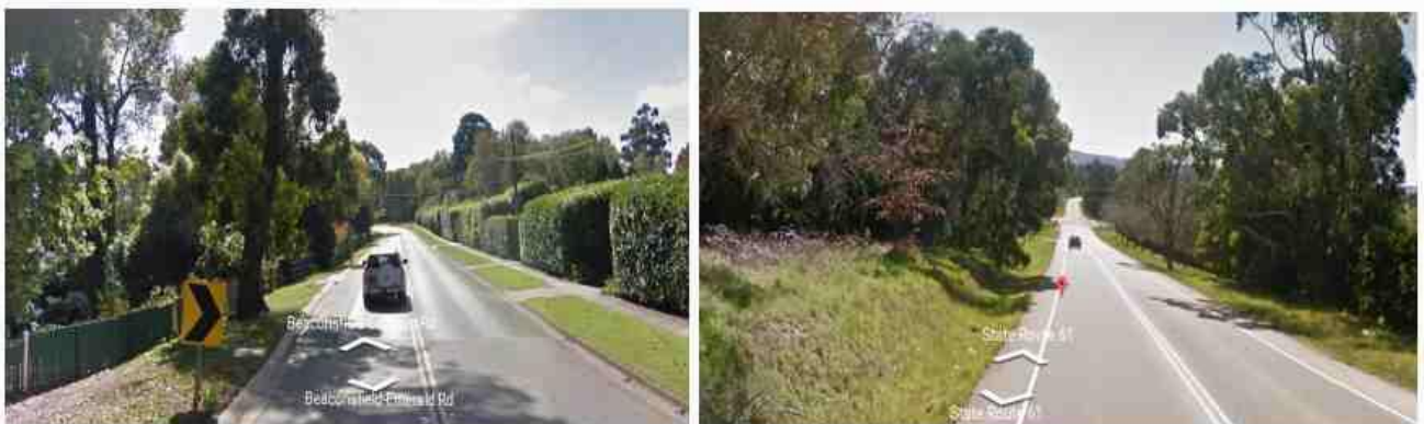
Figure 10: Example of the environments where speed outliers were generated on the test route No2 by the GPS receiver with 10 0 mask angle with speed differences 3.1 km/h (left) and -4.8 km/h (right)
