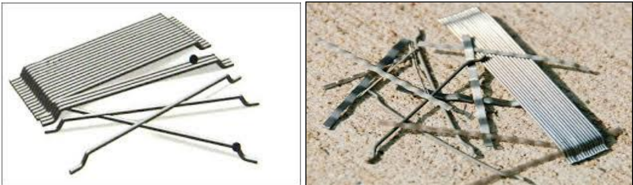
Figure 1. Hook-end Steel Fibre
