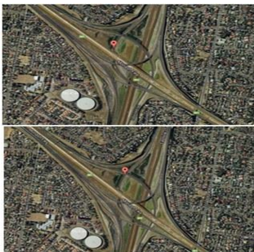
Figure 16: Examples of Environments where the GPS Receiver D generated Speed Spikes
