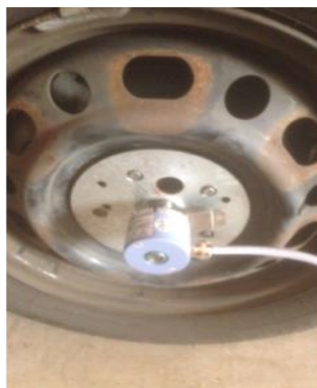
Figure 2: Speed / Distance Sensor Installation
