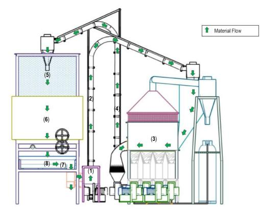
Figure 2. Material flow diagram of the pilot-scale model during dying experiments
