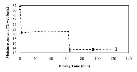
Figure 3. Moisture reduction of paddy dried to fluidized bed dryer at 70°C and 2 min fluidization time with 31% (wet basis) initial MC (error bars  $\pm 0.38$ ).
