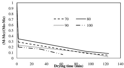
Figure 4. Normalized moisture content of paddy dried to fluidized bed dryer at different drying temperatures with 2 minutes fluidization time.
