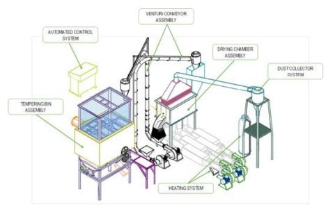
Figure 1. Major components of the pilot-scale model fluidized bed drying system
