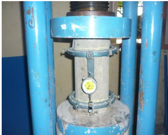
Fig 10. Test set up of Modulus of Elasticity
