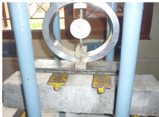
Fig 8. Test set up of prism under Flexural testing machine
