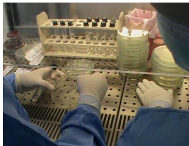
Figure 3. SRB isolation process
