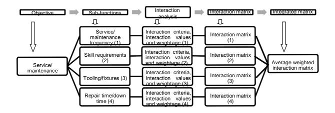
Figure 1: The proposed process flow for interaction analysis for car door service/maintenance objective.
