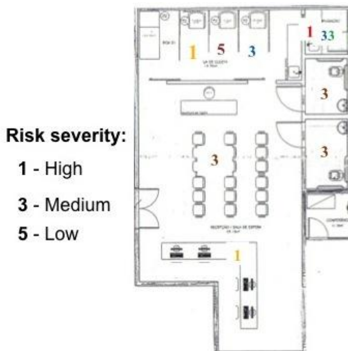
Figure 6. Risk map -Floor plan: numeric indication of severity and the collors of the number indicate risk group
