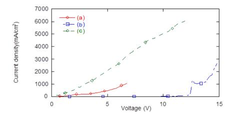
Figure 1 : Current density-voltage plot of, (a) ITO/CdTe type(II)QD/AL (b) ITO- PEDOT/CdTe type(II)QD +Ionic liquid/Ca-Al, and (c) ITO- PEDOT/CdTe type(II)QD+SWNT carboxylic
