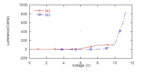
Figure 5 : Luminance-voltage plot of ITO-PEDOT/CdTe Type (II) QD, (a) +0.025mg/ml SWNT carboxylic functionalized/Ca-Al, and (b) +0.0031mg/ml SWNT carboxylic functionalized/Ca-Al
