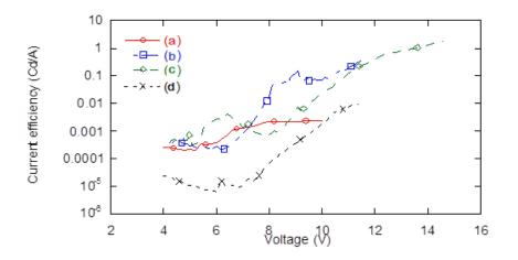
Figure 6 : Current efficiency-voltage plot of ITO-PEDOT/CdTe Type (II) QD, (a) +0.025mg/ml SWNT carboxylic functionalized/Ca-Al, (b) +0.0125mg/ml SWNT carboxylic functionalized/Ca-Al, (c) +0.0062mg/ml SWNT carboxylic functionalized/Ca-Al, and (d) +0.0031mg/ml SWNT carboxylic functionalized/Ca-Al
