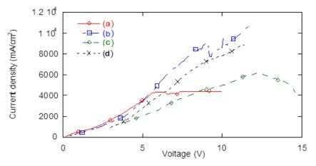
Figure 4 : Current density-voltage plot of ITO-PEDOT/CdTe Type (II)) QD,
