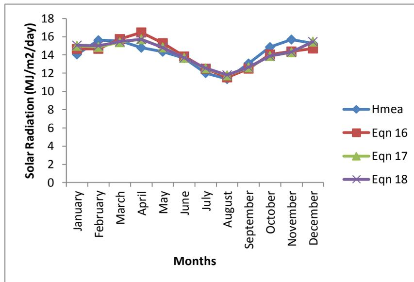
**Figure 2: Comparison between measured and estimated solar radiation using meteorological parameters**
