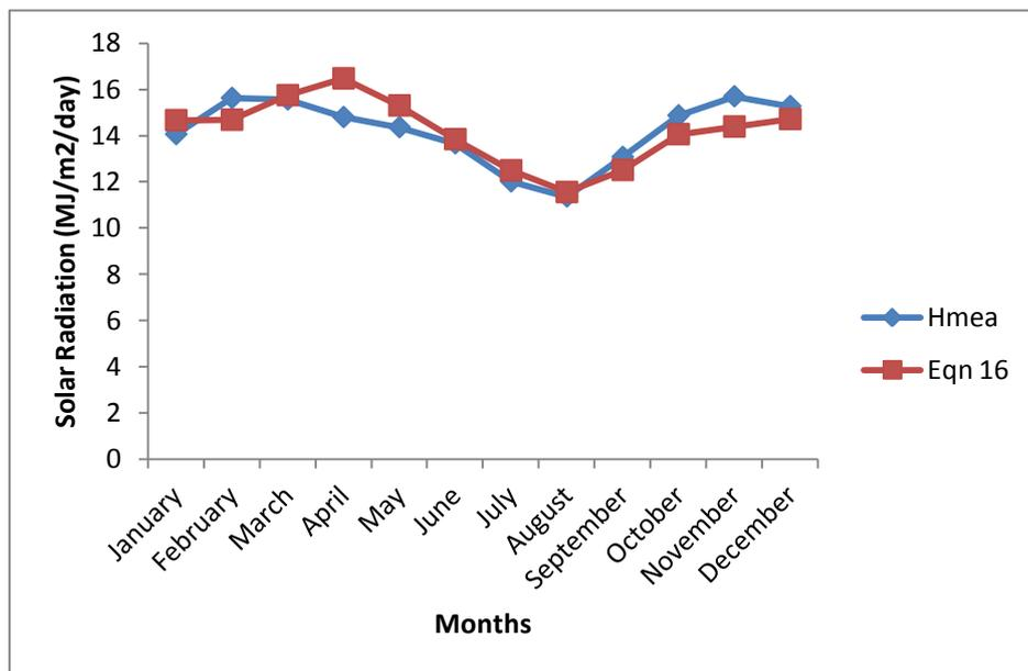
**Figure 1: Comparison between measured and estimated solar radiation using relative sunshine duration hour**
