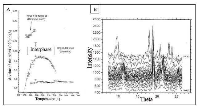
**Figure 4.** A: The d-values of the reflex (020) over the temperature of 270 to 350 K at 10<sup>-3</sup> mbar. And B: Thermodiffractograms of the neutrons scattering experiments of hopeite between 300 K and 500 K in 5 K steps at a pressure of 4.5 mbar.
