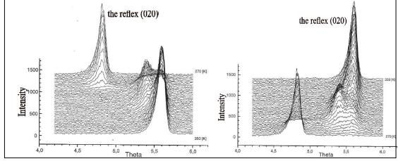
**Figure 2.** The Trend of the reflex (020) between 350K and 270K in 2K steps from 4.2° to 6° Theta and at a pressure of 10<sup>-3</sup> mbar.
