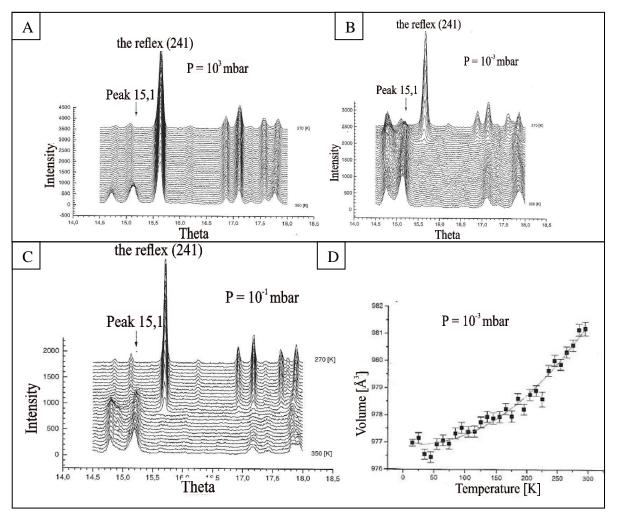
**Figure 3.** A, B, C : Thermal diffractogram of hopeite between 270K and 350K in 3K steps at Theta range from 14.5° to 18° with 10<sup>3</sup>mbar, 10<sup>-3</sup>mbar, and 10<sup>-1</sup>mbar Pressure. And D : Volume of hopeite depending on the temperature between 15K and 295K in 10K steps at a pressure of 10<sup>-3</sup> mbar.
