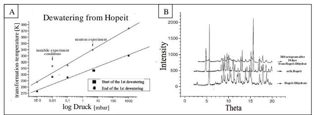
**Figure 5.** A: Graphical presentation of the transformation temperature of the hopeit as a function of pressure. B: Comparison-Diagram of the same sample between an orthorombic-Hopeit and the dihydrat-Hopeit and the Hopeit after 18 days.
