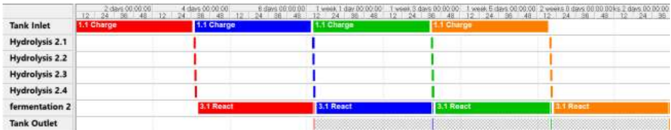
Figure 8: Gantt Chart for the system with 4 tanks of hydrolysis and 1 tank of fermentation.
