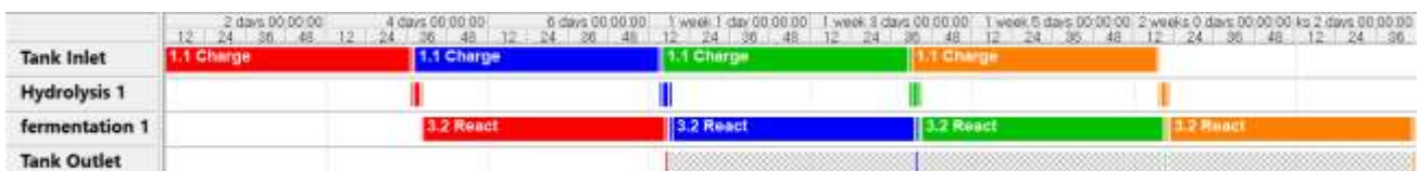
Figure 6: Gantt Chart for the system with 1 tank of hydrolysis and 1 tank of fermentation.
