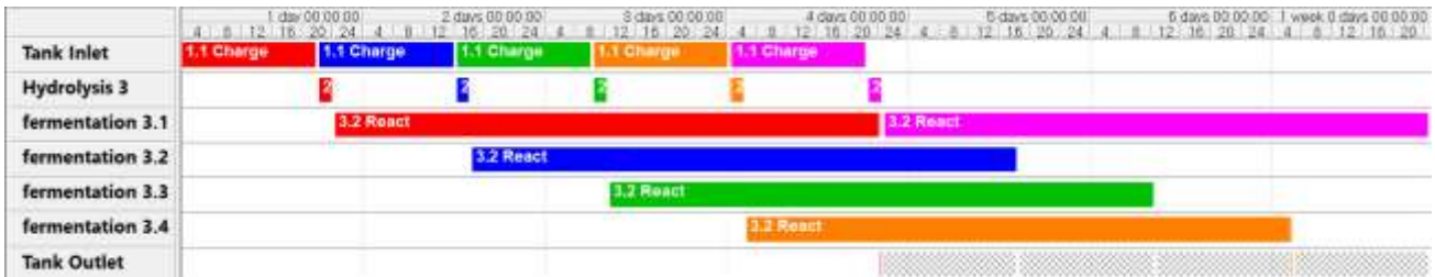
Figure 10: Gantt Chart for the system with 1 tank of hydrolysis and 4 tanks of fermentation.
