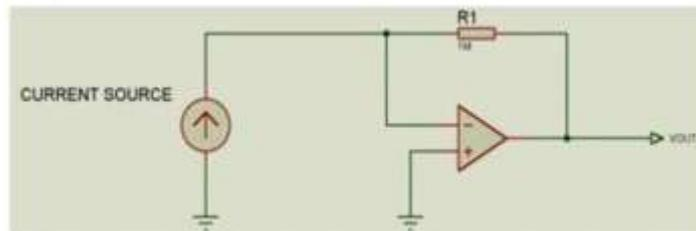
Figure 2: Trans-impedance circuit
