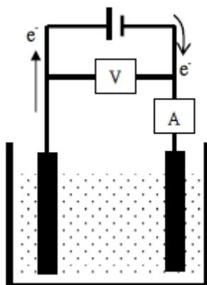
**Figure 1:** Electrochemical circuit of ethanol measurements
