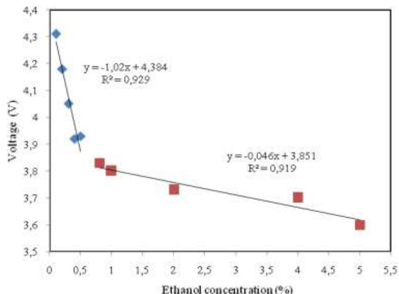
**Figure 5:** Relationship between voltage output of sensor vs. ethanol concentration
