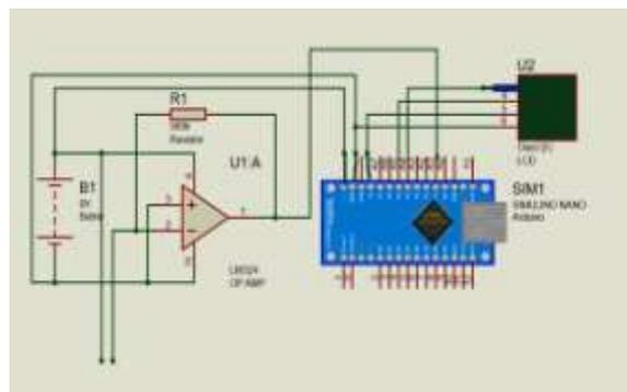
Figure 3: Circuit of ethanol measuring device
