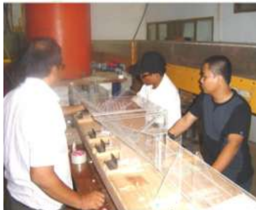
Figure 1: Installation Culvert Model on Observation Table
