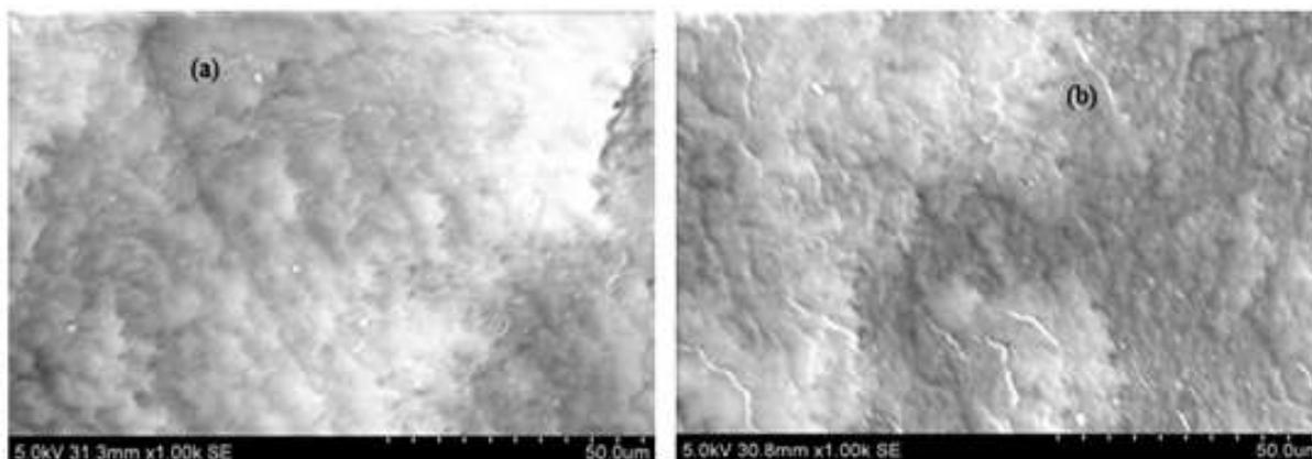
Figure 4: SEM of DNA coated on steel. (a) DNA Alone (b) DNA\_CTMA complex.
