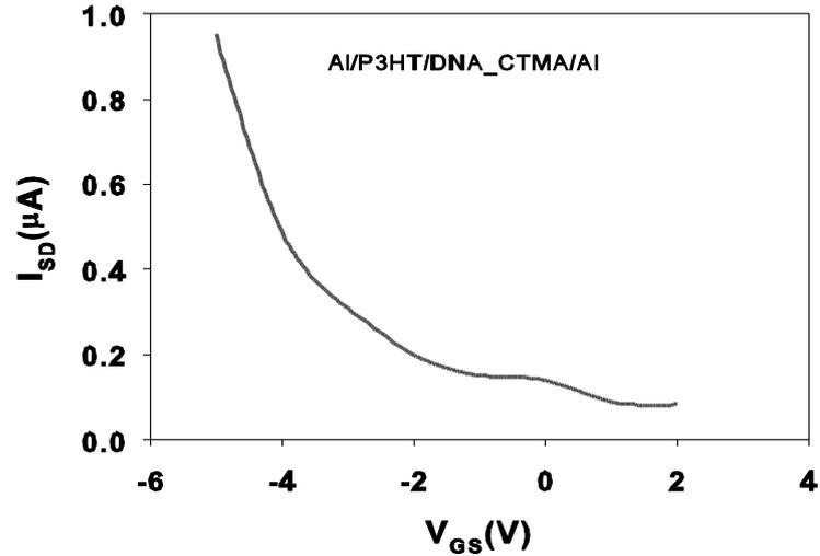
Figure 7: Transconductance curve at  $V_{SD}=10V$
