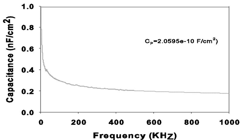
Figure 8: Device frequency versus capacitance curve
