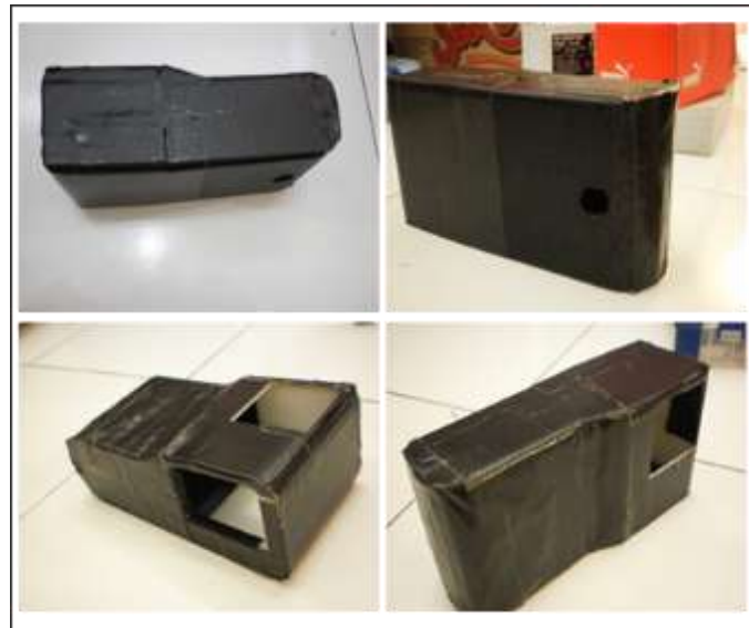
Figure 9 Final Assembly of External Case (using 3D Printers with ABS Plastic Material)
