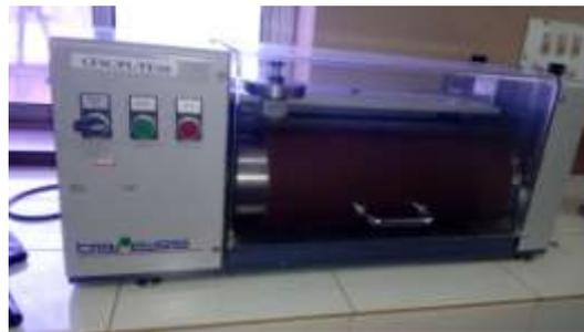
**Fig.2. Rotating drum Abrader.**
