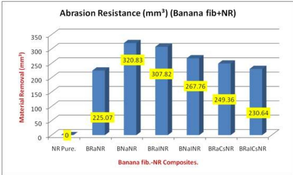
Fig.6. Wear Resistance/ Material Removal rate mm<sup>3</sup>/mm.
