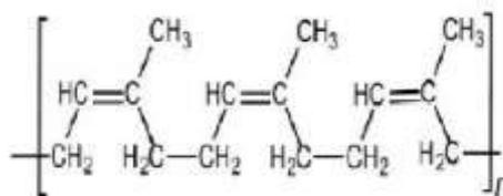
Fig.1. The structure of Natural Rubber.
