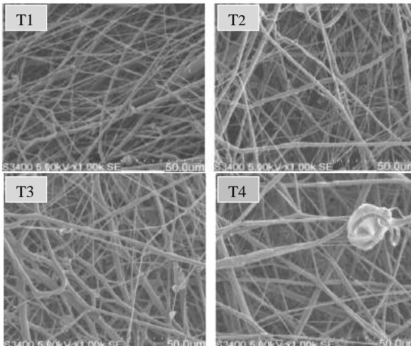
**Figure 2.** Scanning Electron Microscope Images of Electrospun Fibers: (T1) PLA/Chitosan, (T2) PLA/modified  $\alpha\text{-Fe}_2\text{O}_3$  (0.25g) chitosan, (T3) PLA/modified  $\alpha\text{-Fe}_2\text{O}_3$ (0.50g) chitosan, and (T4) PLA/modified  $\alpha\text{-Fe}_2\text{O}_3$ (0.75g) chitosan.
