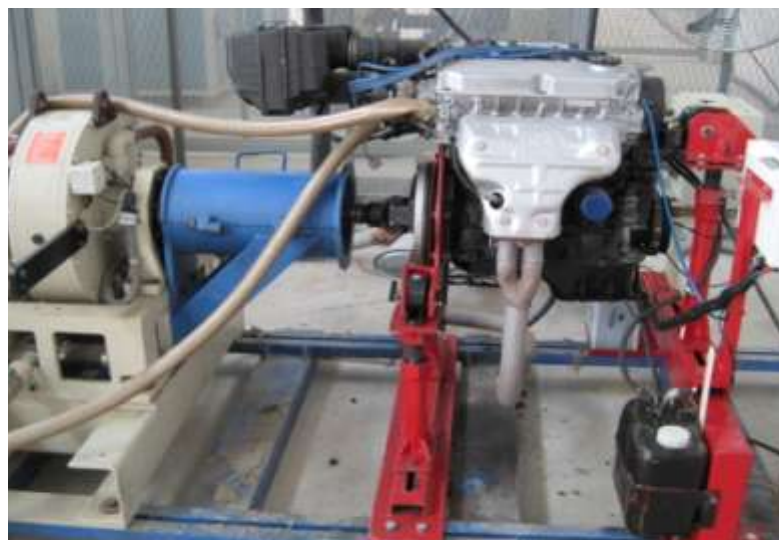
Fig 1. Engine and eddy current dynamometer
