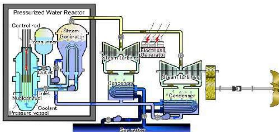
Figure 3, shows the construction of different systems, that there are two steam turbine units [35]
