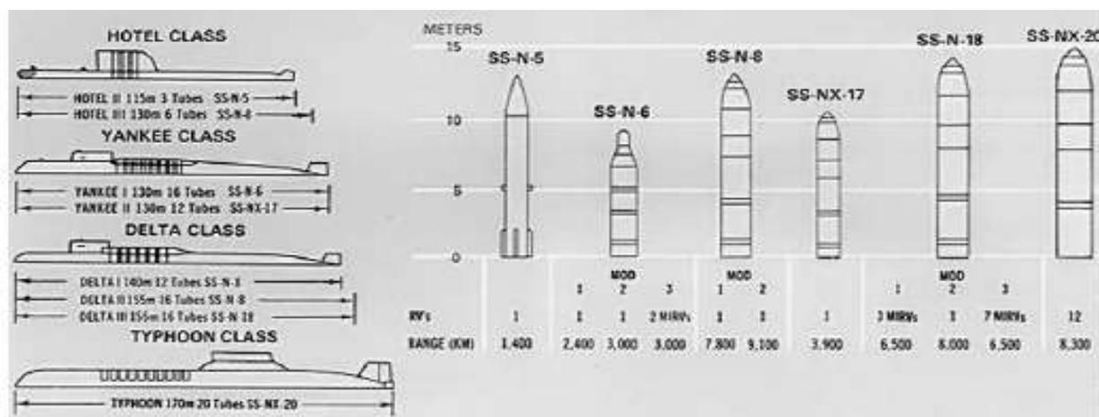
Figure 1. Russian Nuclear Ballistic Missile Submarines and their missile characteristics
