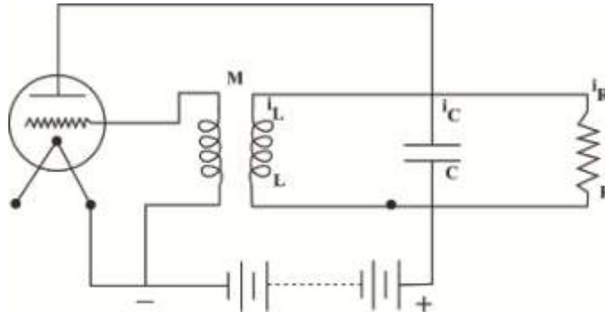
Fig 1: Triode oscillator circuit considered by Vander Pol in obtaining the equation of motion (1).
