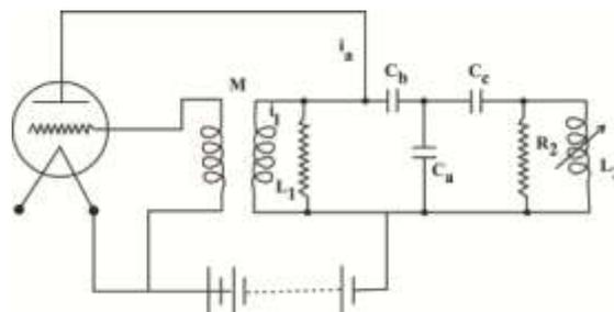
Fig. 2 : double tank circuit considered by Vander Pol in obtaining Eqns (11) and (12).
