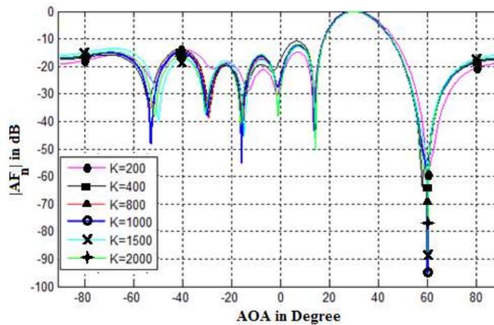
Fig. 8: Normalized array factor using SMI-LMS algorithm for  $d=0.5\lambda$
