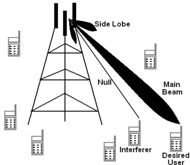
Fig. 2: Main beam toward desired user and null toward interferer
