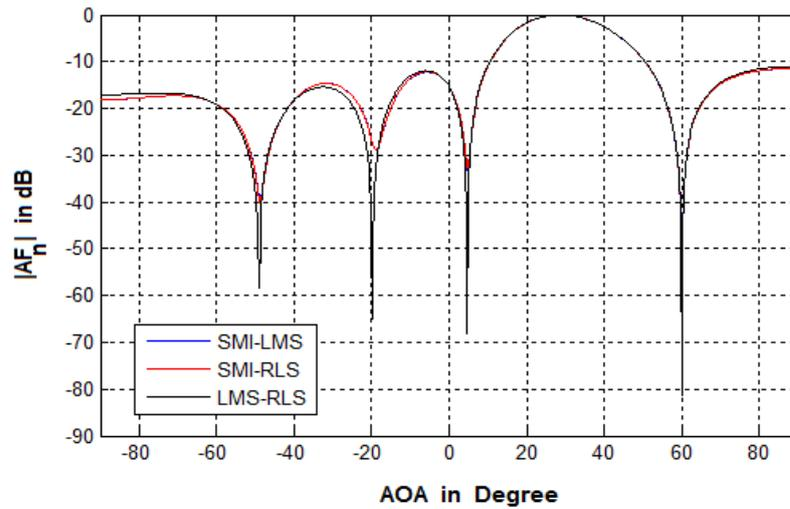
Fig. 6: Normalized array factor for SNR = 20 dB,  $d=0.3\lambda$
