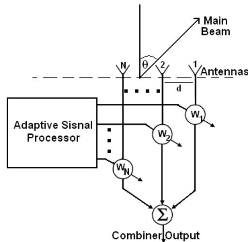
Fig. 1: Beamforming network of a smart antenna
