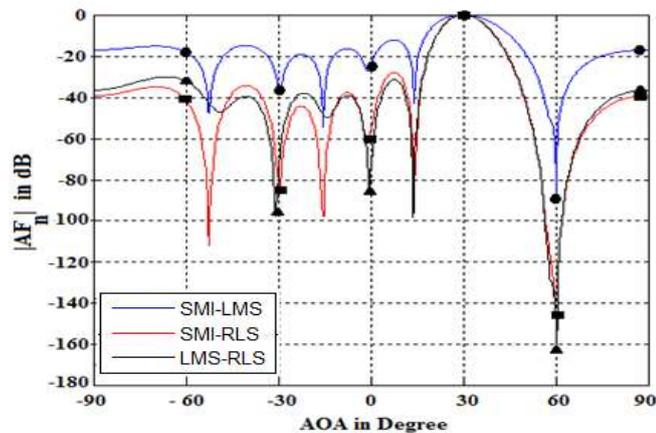
Fig. 4:Normalized array factor for SNR=20dB and  $d=0.5\lambda$
