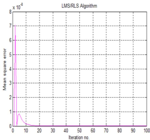
Fig. 12: Mean square error for 8 elements linear array using LMS-RLS algorithm
