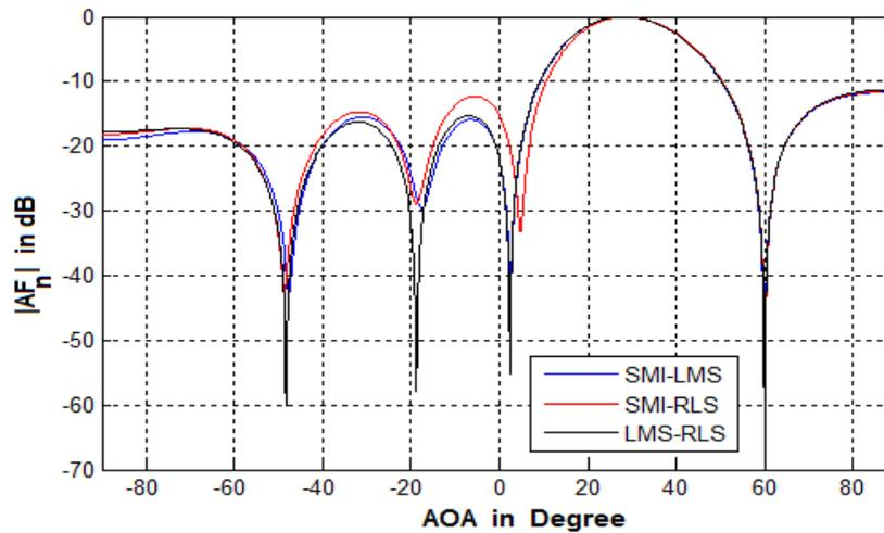
Fig. 7: Normalized array factor for SNR = 10 dB,  $d=0.3\lambda$
