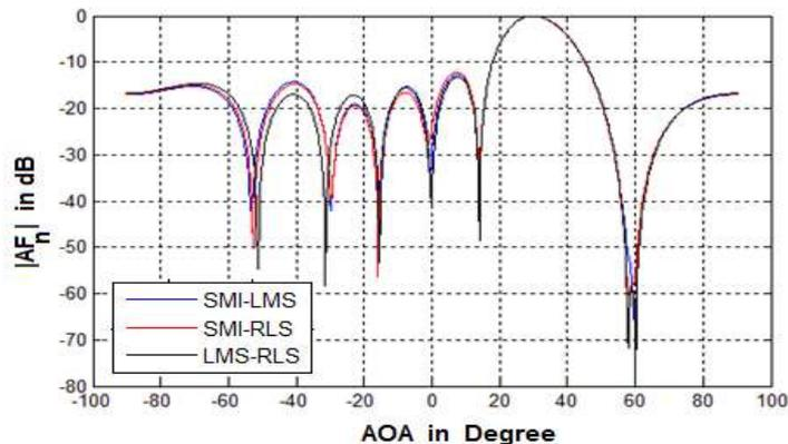
Fig. 5:Normalized array factor for SNR = 10dB,  $d=0.5\lambda$
