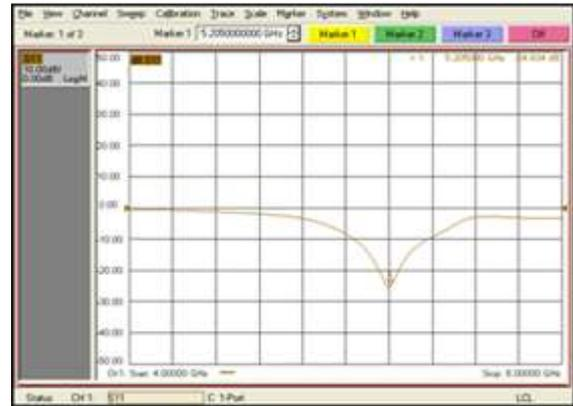
Figure 4: Measured Return Loss
