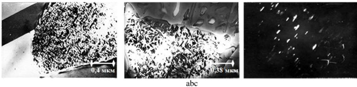
Fig.6. The microstructure of the particles within the decay  $\alpha$ -phase after quenching from 1250<sup>0</sup>C, 1 min. and aging: a - 600<sup>0</sup>C, 10 hours, x24000; b - 700<sup>0</sup>C 5 hours, x26000; c - darkfield image structure in Fig. 6b.
