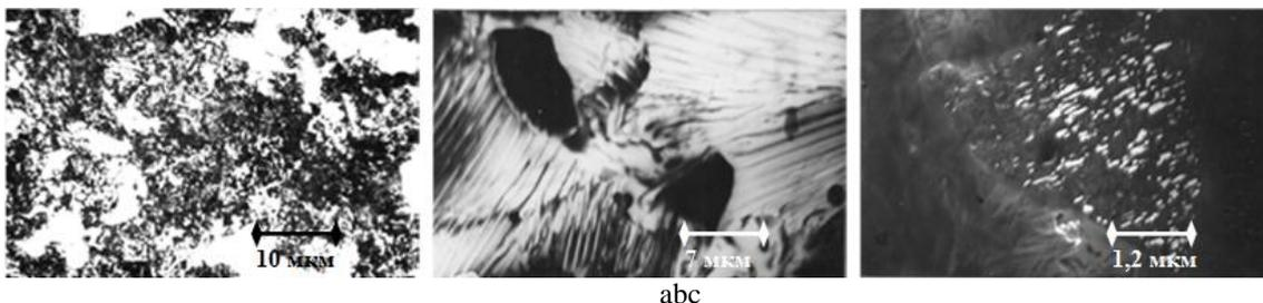
Fig.1. Microstructure of tempered 1250°C, 1 min. 47CrNiMo alloy after aging at 800°C, 2:00 hours a - x1000; b - x1300; c - x8500
