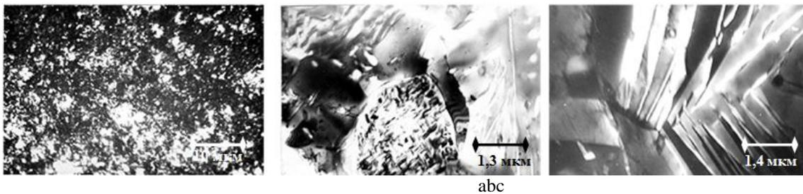
Fig.2. The microstructure of the alloy aged at 900°C 1250°C from pre-hardened, 1 min: a - x1000; b - x7500; c - x7000
