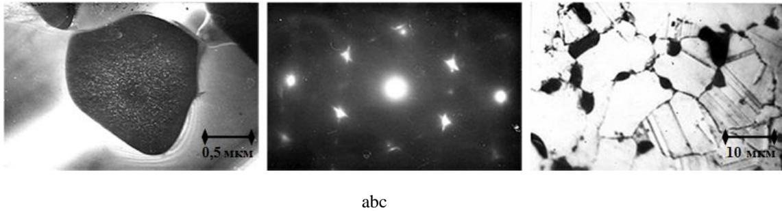
Fig.5. The structure of globular particles  $\alpha$ -phase after quenching from 1250<sup>0</sup>C, 1 min. and aging at 600<sup>0</sup>C, and 2 hours: dark-field image strands  $\alpha$ -phase x18500; b –optical photomicrography the structure shown in Fig. 5a; c - an optical micrograph, x1000
