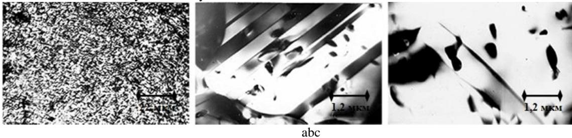
Fig.3. The microstructure of the alloy after quenching from 47CrNiMo 1250°C, 1 min. and aging at 1000°C: a - 5 hours, x450; b - 1 hour, x8500; c - 1 hour, x8500
