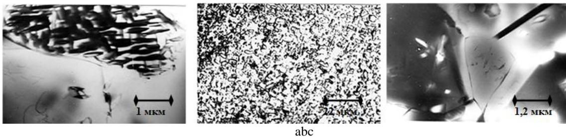
Fig.4. Microstructure of pre-hardened by 1250°C, 1 min. alloy after aging: a - 1000°C 0.1hours, x10000; b - 1100°C 0.5 hours, x450; c - 1100°C, 1 hours, h8000
