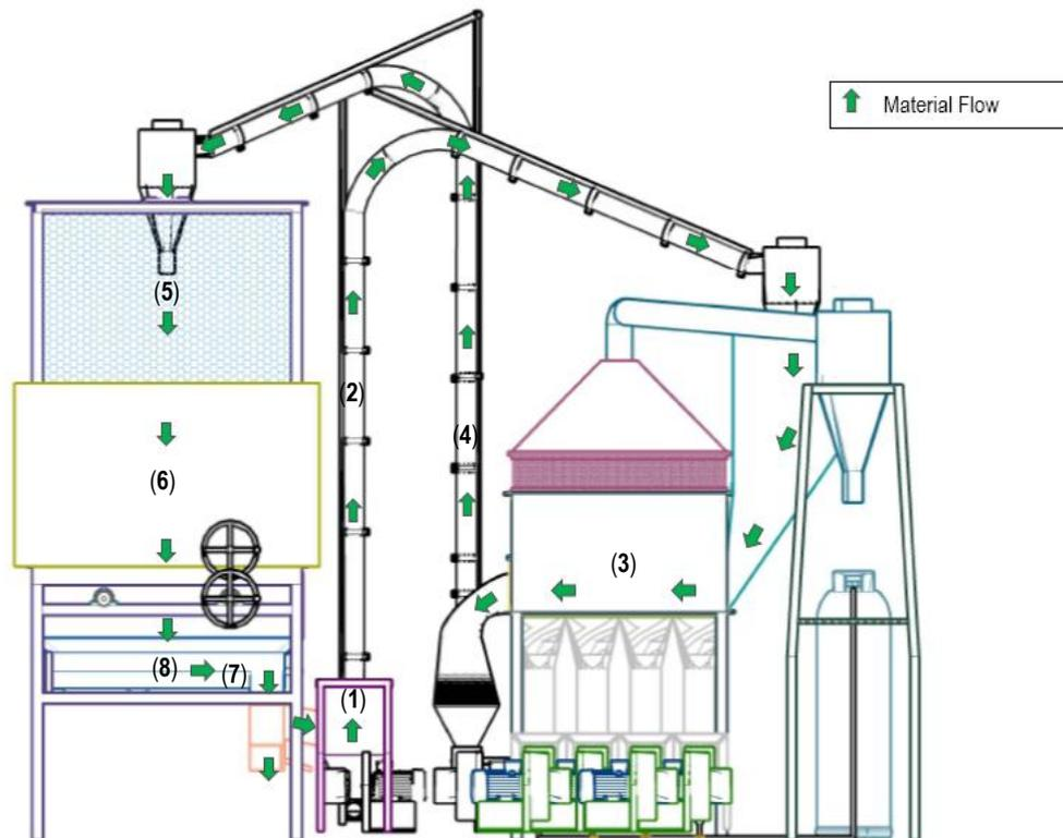
**Figure 2.** Material flow diagram of the pilot-scale model during drying experiments
