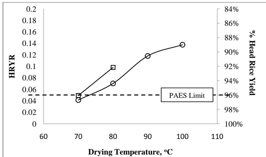
**Figure 6.** Head rice yield reduction ratio of samples dried in the pilot-scale fluidized bed dryer in relation to the different drying temperatures
