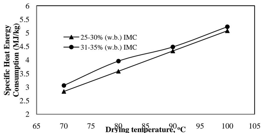
Figure 5. Specific heat energy requirement (MJ/kg) of paddy dried using the pilot-scale fluidized bed dryer at different drying temperatures with 2 min fluidization time and 60 min tempering period.
