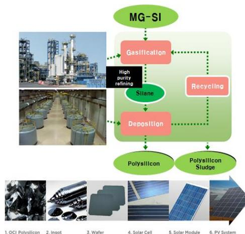
Figure.1 Polysilicon Production process
