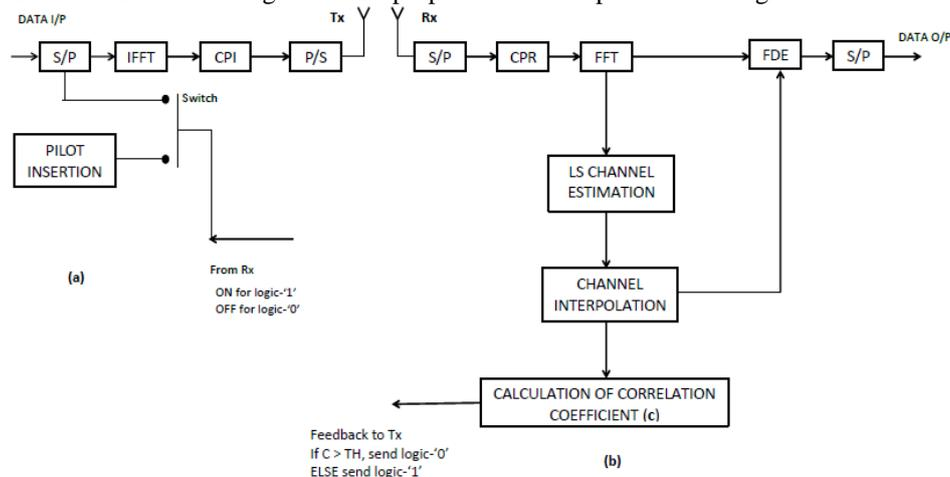
Fig. 1. Proposed system model, CPI: Cyclic prefix insertion, CPR: Cyclic prefix removal, FDE: Frequency domain equalizer
