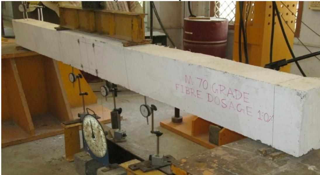
Figure .3 Test Set- Up and Instrumentation
