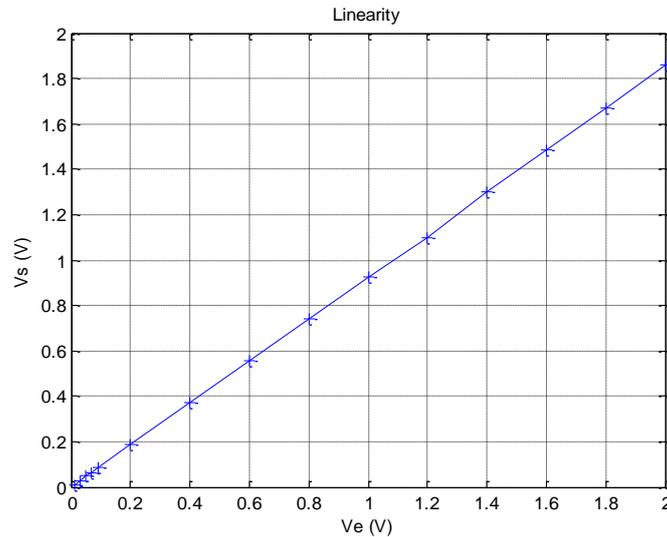
**Fig. 9** Measured Nonlinearity for one channel.
