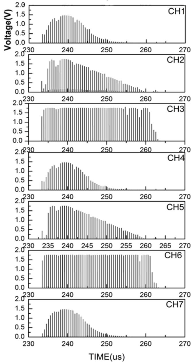
Fig. 7 Simultaneously analog output reconstruction for 7 channels
