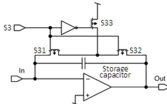
Fig.3 A T-Network configuration as the reset switch.
