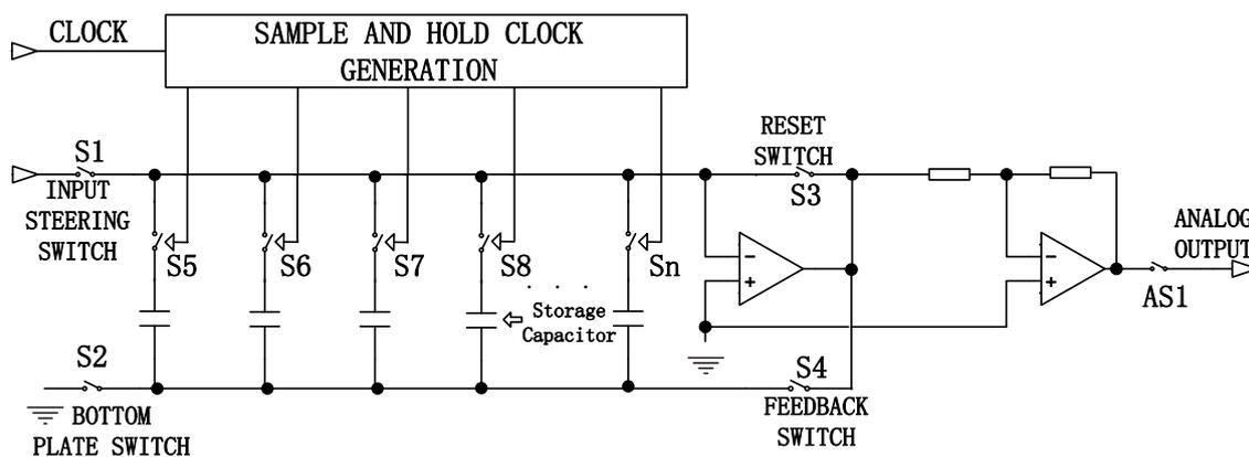
**Fig. 1:** Simplified circuit of a single channel.
