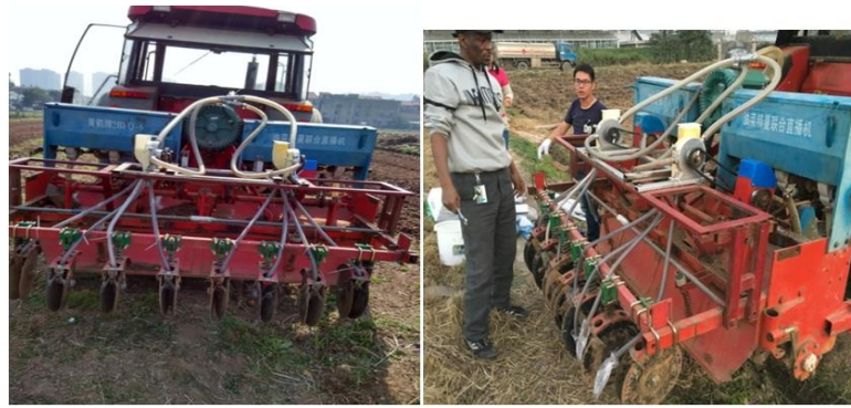
Figure 4: Two copies of the prototype mounted to a seed planter for field experiment.
