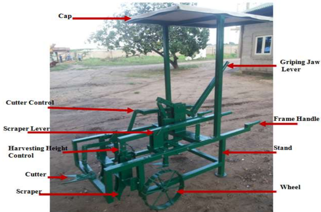
Figure 1: The Cassava Harvester and Stem Cutter
