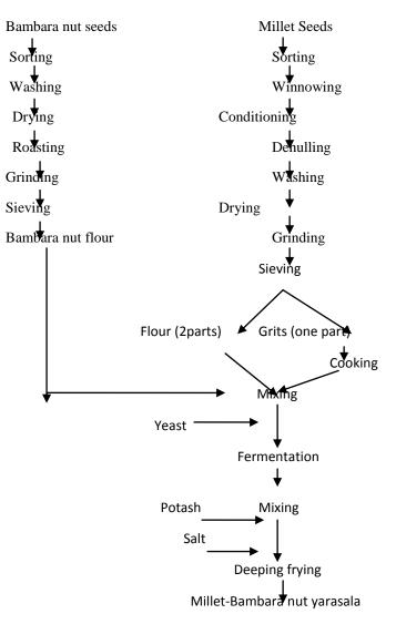
Fig.1: Flow chart for the production of *yar'tsala* made from millet – Bambara groundnut flour blend.
