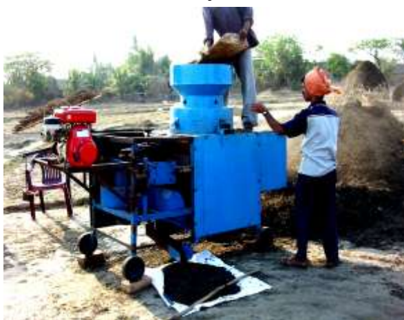
Figure 6: Operation of Automatic Vertical Flow Pulse Thresher
