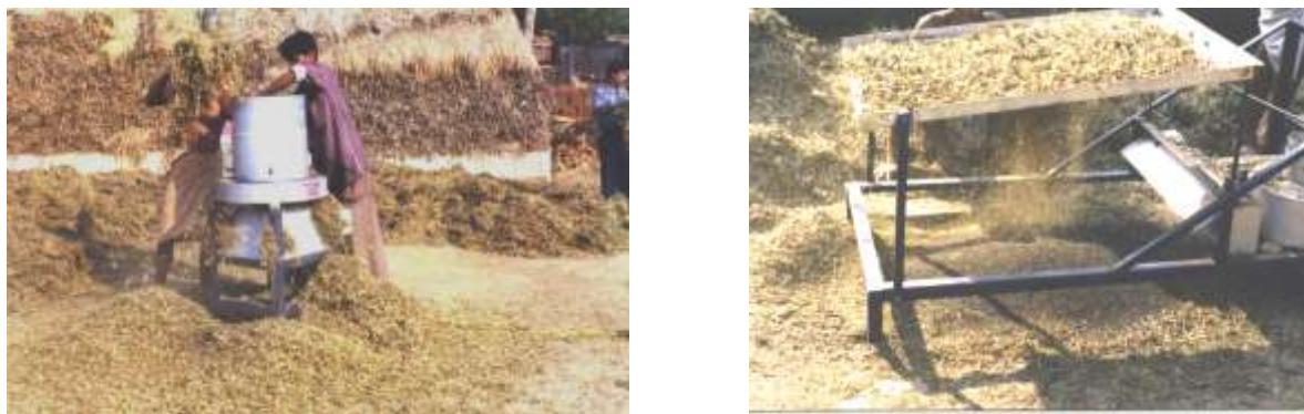
Figure 5: Threshing and Winnowing by Pulse Thresher
