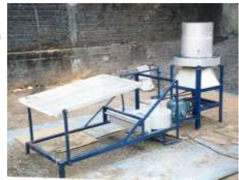
Figure 4: Semi-automatic Vertical Flow Pulse Thresher- cum- Winnower
