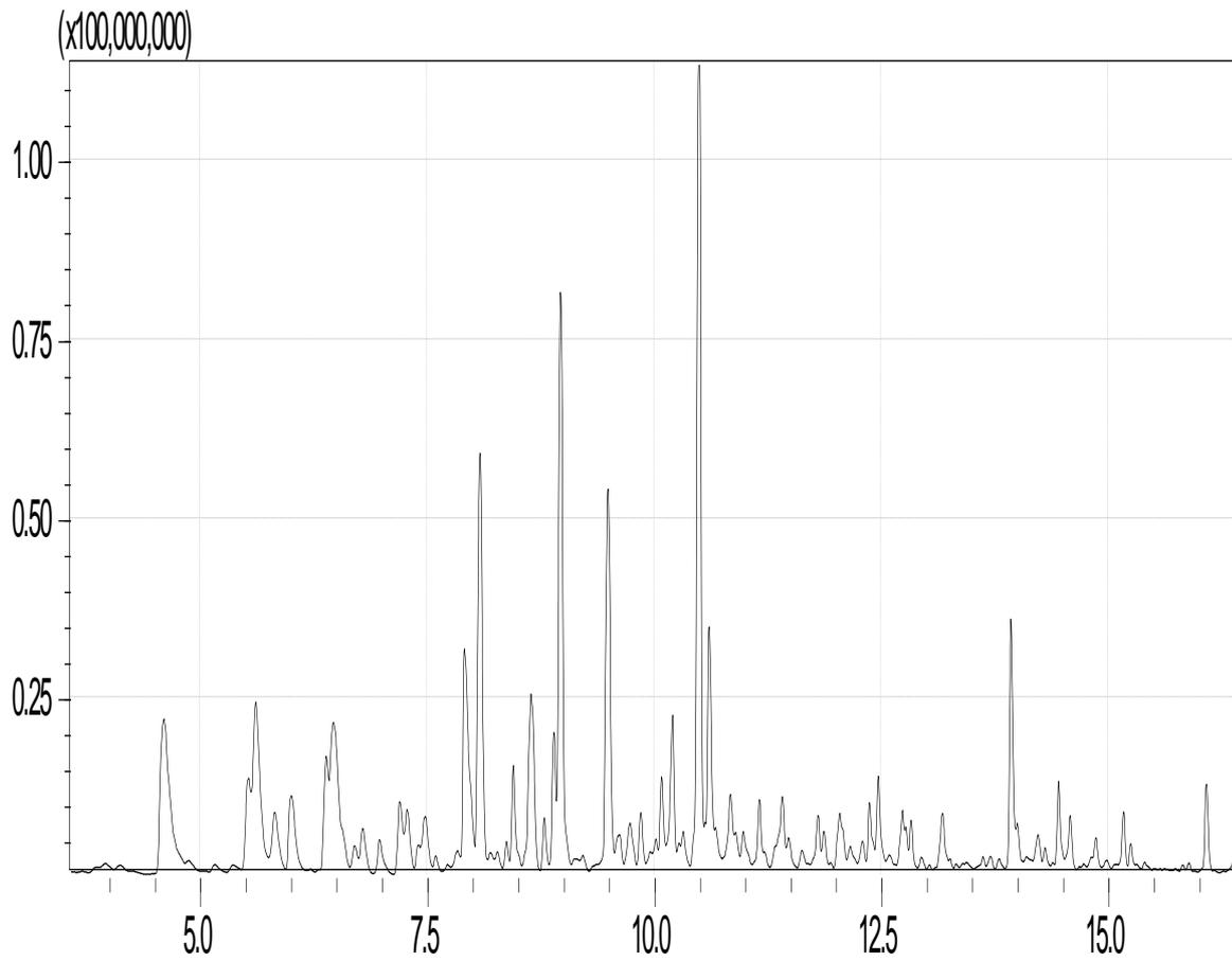
**Figure 1:** Chromatograph of aroma profiles of roasted coffee analysed by SPME/GC-MS
