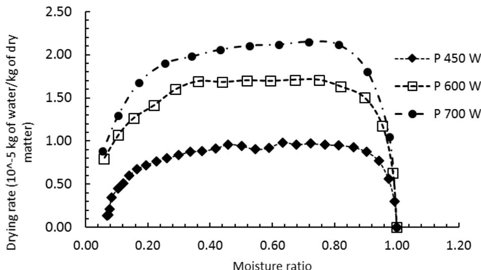
**Figure 2:** Variation of drying rate with moisture ratio at different microwave powers
