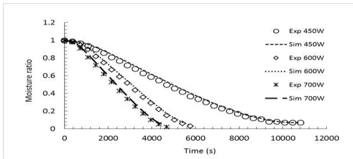
Figure 3: Diffusion model simulation for various microwave powers levels.
