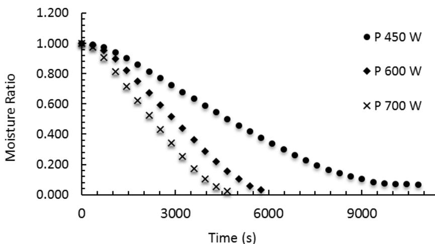
**Figure 1:** Variation of cocoa beans moisture ratio with drying time at different microwave powers
