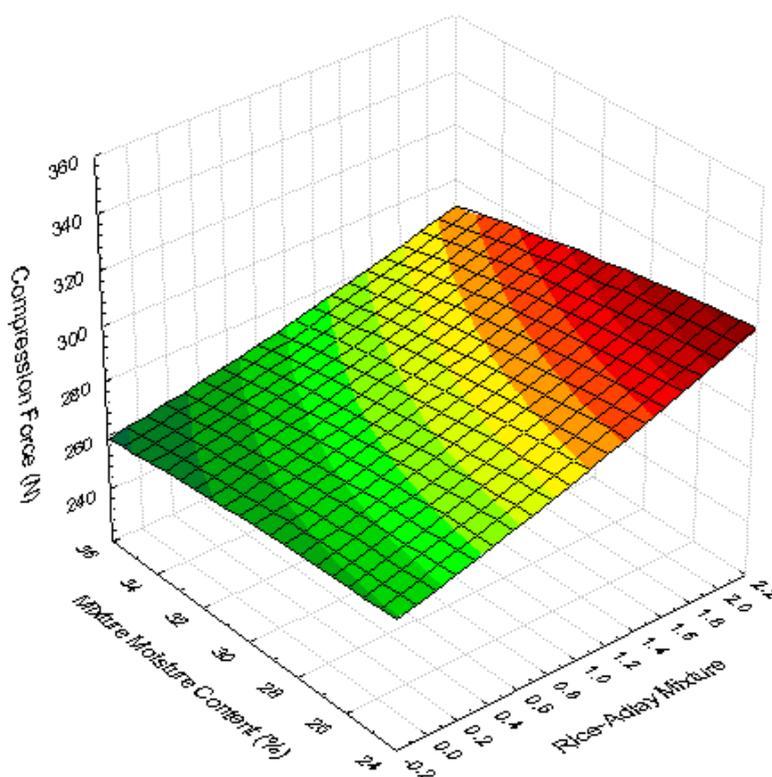
**Figure 2.** The interaction effect of mixture moisture content and rice-*adlai* mixture on compression force.
