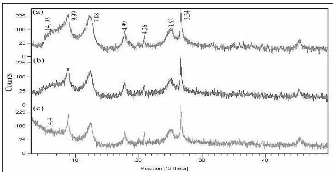
**Figure 5:** X-ray diffraction pattern for treated clay sample from Bs horizon of Jerijeh 2; (a) untreated sample, (b) Mg-saturated, and (c) Mg-saturated, glycolated.
