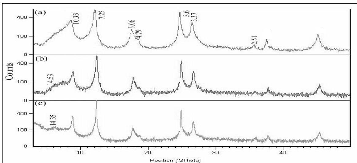
**Figure 3:** X-ray diffraction pattern for treated clay sample from Bhs horizon of Jerijeh 1; (a) untreated sample, (b) Mg-saturated, and (c) Mg-saturated, glycolated.
