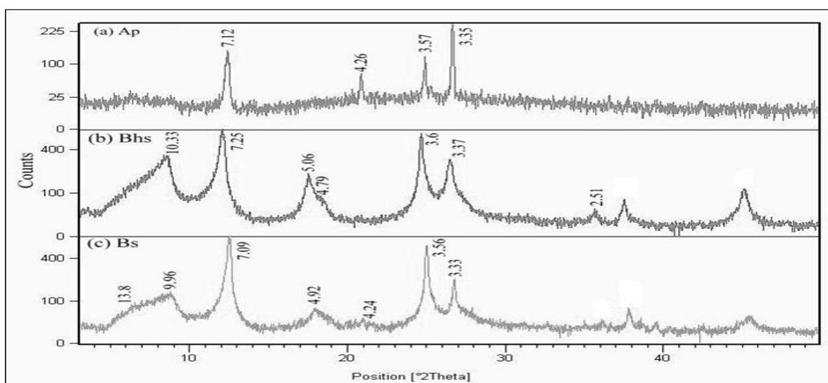
**Figure 1:** X-ray diffraction pattern for untreated clay sample from Jerijeh 1.
