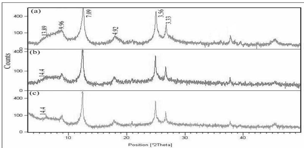
**Figure 4:** X-ray diffraction pattern for treated clay sample from Bs horizon of Jerijeh 1; (a) untreated sample, (b) Mg-saturated, and (c) Mg-saturated, glycolated.
