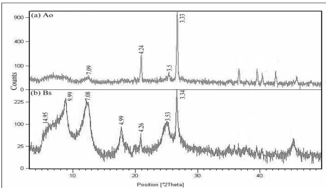
**Figure 2:** X-ray diffraction pattern for untreated clay sample from Jerijeh 2.
