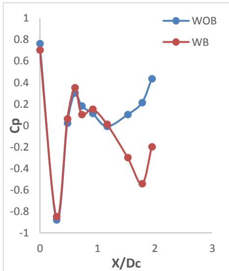
Figure 5 pressure recovery comparison
