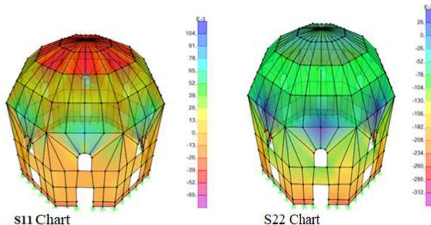
Figure 3. G loading S11 (X direction) and S22 (Y direction) tensile distribution ( $10^{-3}$ N/mm<sup>2</sup>)
