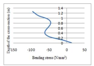
Figure 11: Bending stress distribution of curved Igirder without stiffeners
