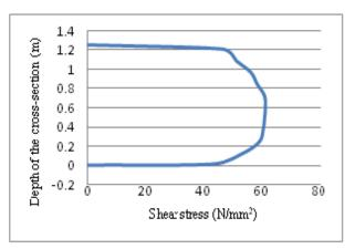
Figure 10: Shear stress distribution of straight I-girder
