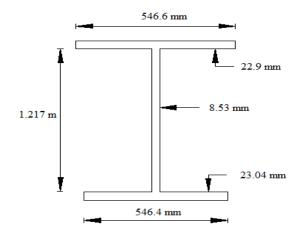
Figure 1: Cross-section of the I-girder
