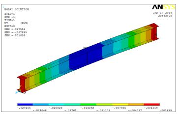
Figure 7: Contour plot of the vertical deflection of curved I-girder with one intermediate stiffener
