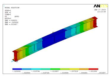
Figure 8: Contour plot of the vertical deflection of curved I-girder with three intermediate stiffeners
