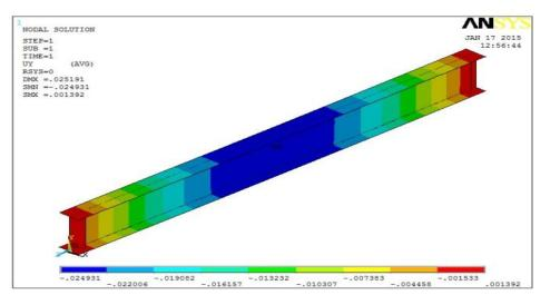
Figure 5: Contour plot of the vertical deflection of straight I-girder
