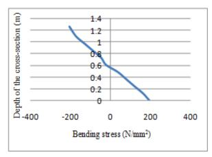
Figure 9 : Bending stress distribution of straight Igirder
