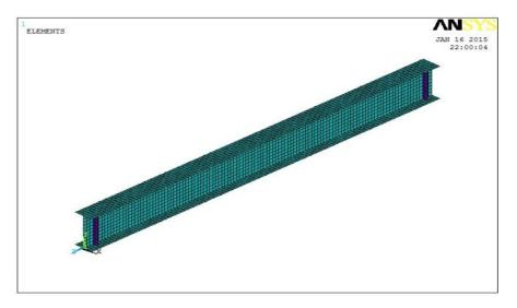
Figure 3: Meshed model of the straight I-girder
