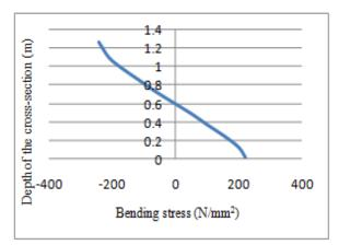
Figure 13: Bending stress distribution of curved Igirder with one intermediate stiffener
