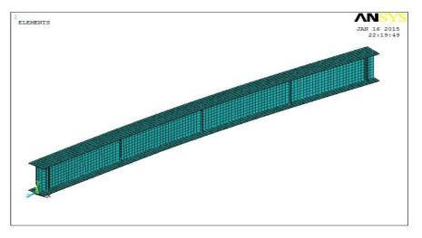
Figure 4: Meshed model of the curved I-girder with three intermediate stiffeners
