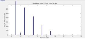
Figure 2: FFT Analysis without filter
