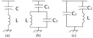
Figure 1: Different Filter Topologies (a) ST Filter (b) C Type Filter (c) CCL Filter [5]
