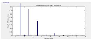
Figure 4: FFT Analysis of source current with single tuned filter
