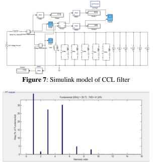
Figure 8: FFT Analysis of source current with CCL filter
